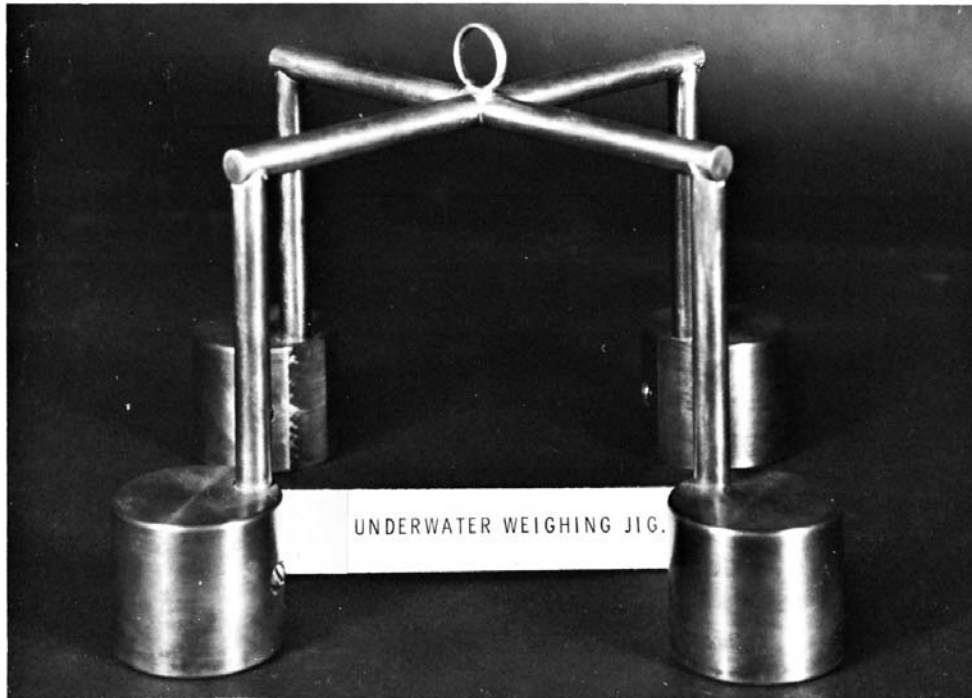
FIG. 1 Underwater Weighing Jigs
